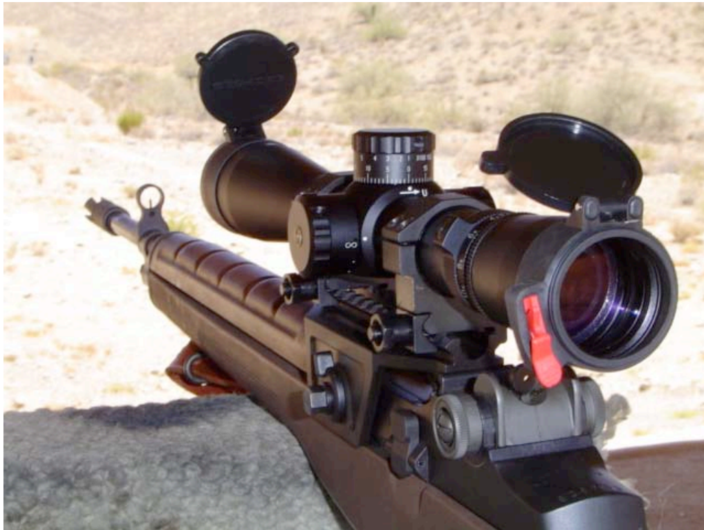
Fig. 1 Smith Enterprise, Inc. US Army (2ID) issue M-14SE with standard Leupold Mark 4 3.5-10X40 LR/T M3 Telescopic Sight.
