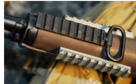
Picatinny rails mounted at 3, 6, and 9 o'clock positions on rifle fore-end.
