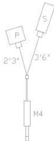
Figure 6. Polaroid and Video Camera Setup - Front View
